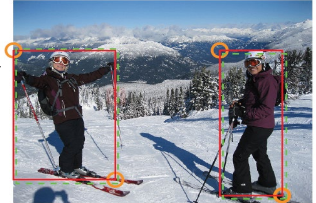
Fig. 5 “Ground-truth” heatmaps for training. Boxes ( green dotted rectangles ) whose corners are within the radii of the positive locations ( orange circles ) still have large overlaps with the ground-truth annotations ( red solid rectangles ).
