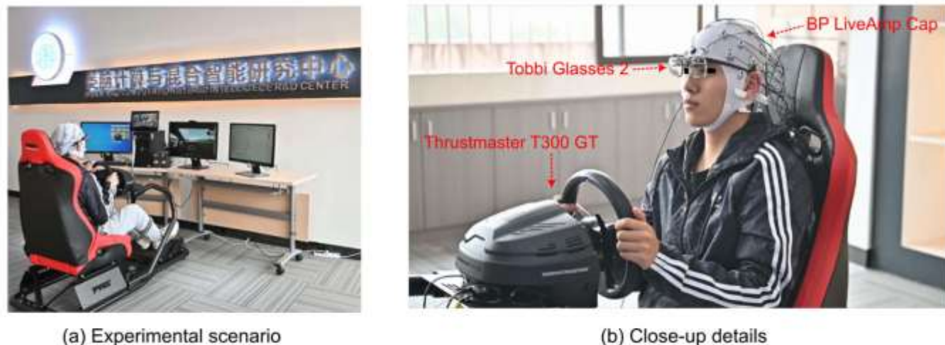
Fig. 1. The system of multimodal driving fatigue detection. (a) experimental scenario. (b) a subject wearing an EEG cap and a pair of Tobii Glasses was driving a simulated vehicle in the simulation platform.
